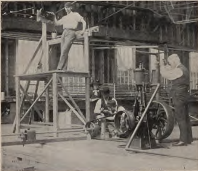
Fig. 37.—Marking off the dynamometer. In order to ascertain the actual amount of power consumed in driving the propeller, a brake was put on in place of the screw, a weight applied, and the engine run at full speed. In this way all the uncertain and unknowable factors were eliminated.
